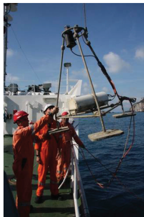
Figure 48. Deployment of a LOON tripod.
