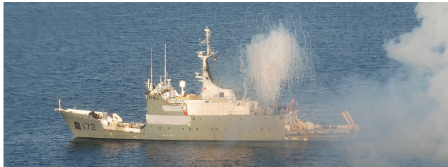
Figure 20. The Canadian Forces Auxiliary Vessel (CFAV) Quest , a Research Vessel, Deploying IR Decoys.
