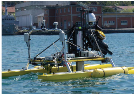
Figure 27. The Gemellina ASV poised to launch the Goldrake 'slave' package. Repeated successful remote-guiding missions were accomplished during the ANT'12 experimentation from 28 May through 18 June and from 17 October through 4 November 2012.
