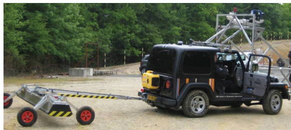
Figure 3. Vehicle with Towed Ground-Penetrating Radar and Several Electro-Optic Detection Systems.
