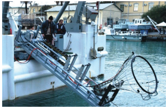
◀ Figure 49. AutoLARS design and during at-sea trial.
