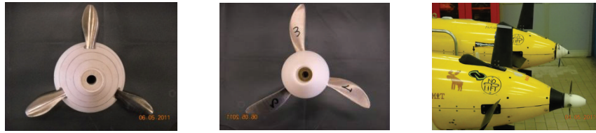
Figure 46. OEX-C original propeller design (left) and the new design (right).
