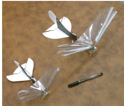
➤ Figure 5. MAV Data Collection: TU Delft DelFly III Marked with Reflective Tape and Hemisphere Markers; Wright State University (WSU)
