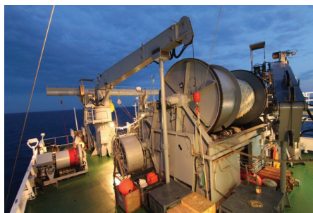
Figure 30. Aft deck of the NRV ALLIANCE with winch for Low Frequency Active (LFA) Variable Depth Sonar (VDS).
